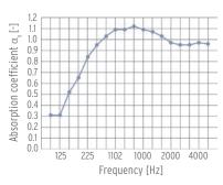
\*The absorption factor (alpha value) indicates how large the absorbed portion of the incident sound is. It is given in the range O-1, where e.g. 1 stands for an absorption of 100%.
