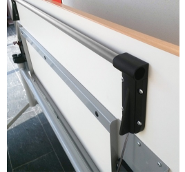
Triggering of the folding function by means of 2-hand safety operation
