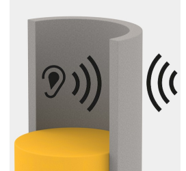
Sound insulation through sound absorbing foam in backrest
